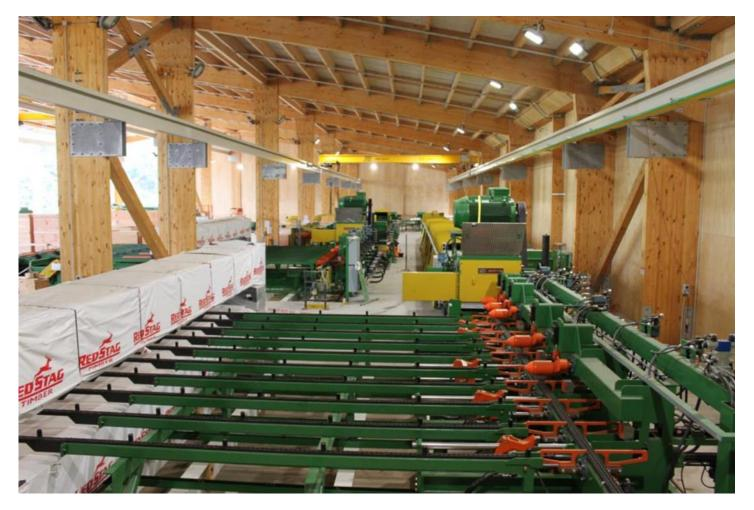
Rotorua based Red Stag sawmill being constructed in 2016. USNR equipment. Note the use of NZ Radiata pine Engineered Wood Products in the 110 metre long sawmill building
